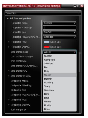
All profiles arranged automatically on chart right margin. Increase margin value in chart properties to free more space for Stacked profiles.
