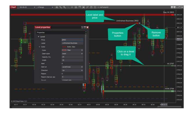
When adding a level click inside Footprint bar or Volume profile/TPO to set this visual as a sarting point of the level. See image.
